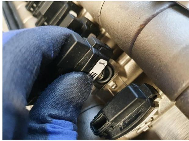
4. Remove the sensor by pulling it out
