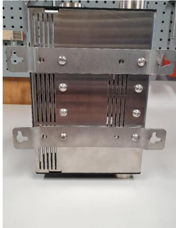
3. Mount the brackets by using the same screws which were just removed. Beware that the bracket should be mounted so the holes at the ends point “upwards” as on the picture. If the holes are pointing “downwards”, then the manifold can still be mounted, if you turn it upside down.
