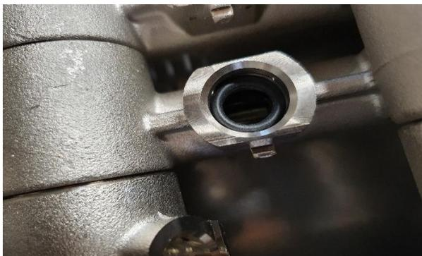
5. Make sure that the sensor is removed correctly. Remove anything from the pipes, like the O ring which commonly gets stuck.
