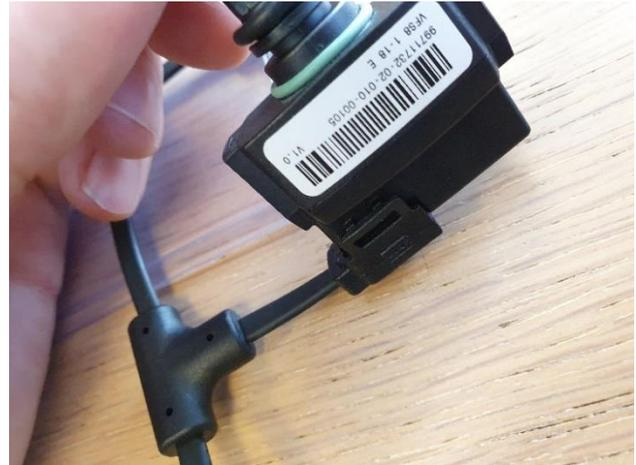
6. Place the sensors, so they rest on the cable, and ensure that the sensors and cable are aligned.
