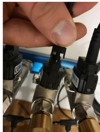
3. Once both sides are released from the snap fit, you can pull out the sensor gently
