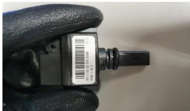
6. Replace sensor if needed, and remount the O ring if it fell off in step 5.
