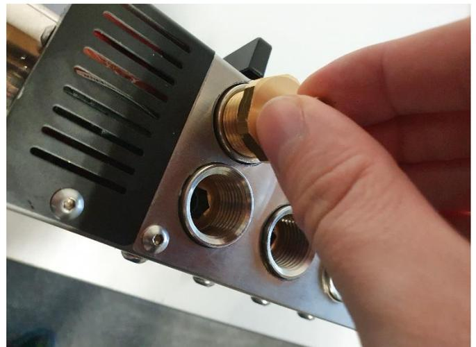
1. Select fittings appropriate for your needs. Remember to have an appropriate O ring on the fitting. The thread in the channels is G 1/2".
