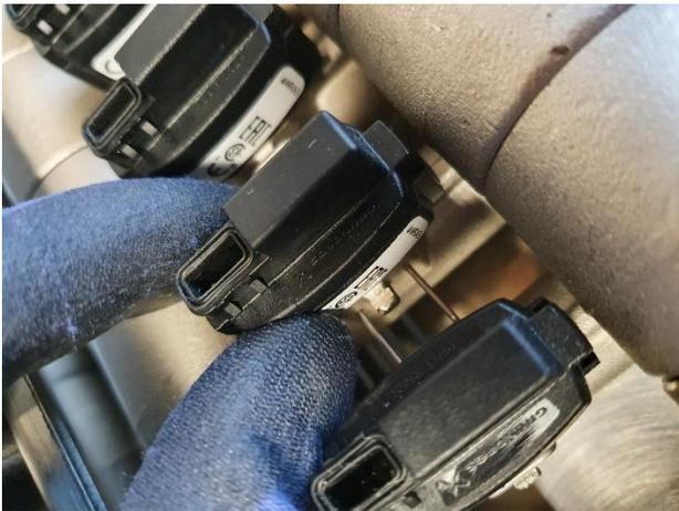
3. Once the pin is pulled out far enough, the sensor is no longer locked in place.
