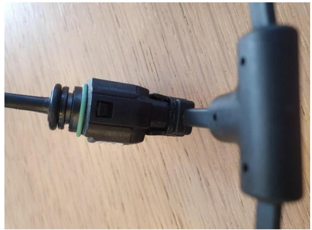
8. Make sure that the snap fits on both sides lock the sensor. Do this for all sensors and cables.
